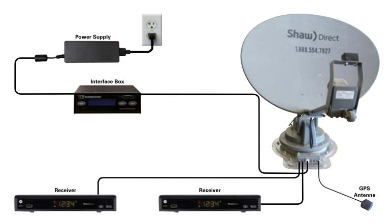
FIGURE 8. Setup with fully assembled antenna
