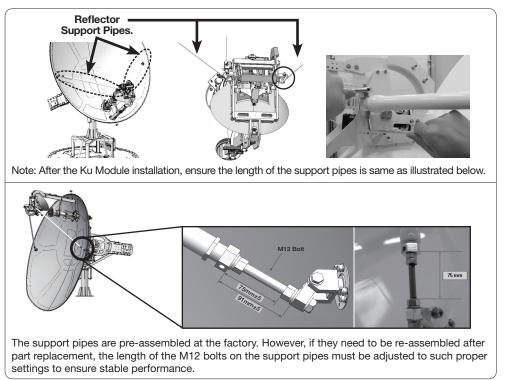
Ku Module and Reflector Support Pipes
