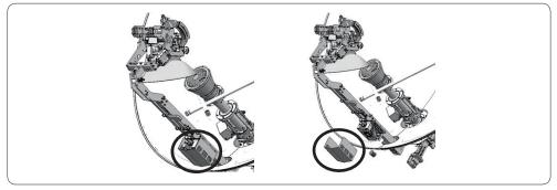
Ku Module Cover Removal (For Circular and Linear Model with a Ku-band BUC on Support Pipe)
