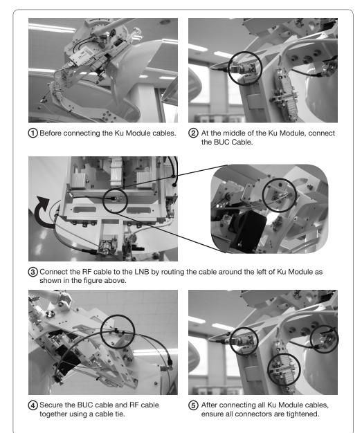
**Ku Module Cable Connections**
