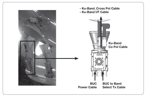
For a Circular and Linear system with a Ku-band BUC on the support pipe, connect the cables and clean up using cable ties as shown below.
