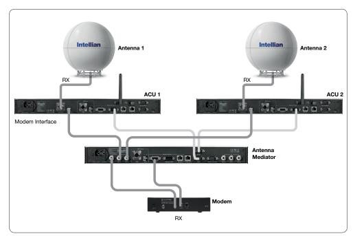
System Configuration RX: 2 Antennas and 1 Modem
