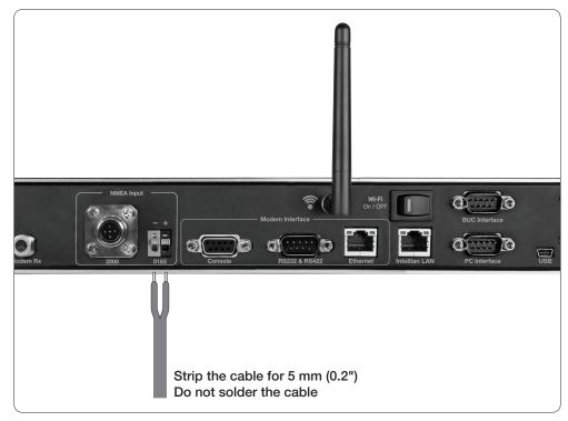
Ship's Gyrocompass Connection
