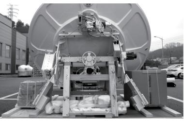
ACU, Installation Kit Box, Ku Module Box, Ku Module Support Pipe, and EL Support Frame
