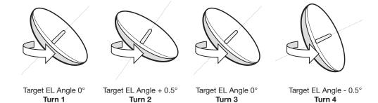
Search 3: a search pattern 3 automatically initiates when the AGC / SIG falls below the current tracking level threshold value. If the desired signal is found and above the predefined tracking level, the ACU will terminate Search 3 and go into TRACKING mode.
