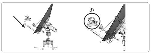
Connect Ku Module and Ku Module Support Frame
