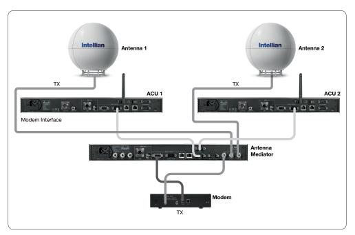
System Configuration TX: 2 Antennas and 1 Modem
