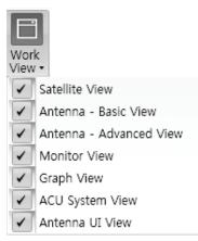
Work View: displays a list of seven pre-constructed Work View Tabs (Satellite View, Antenna Basic View, Antenna Advanced View, Monitor View, Graph View, ACU System View, and Antenna UI View) and also provides the Activate / Close functionalities for each view tab. Activate the work view tab by ticking the checkbox next to it.
