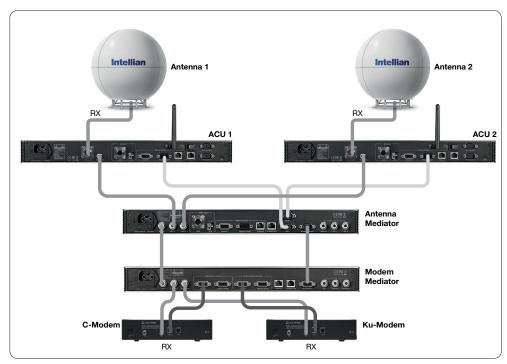
System Configuration RX: 2 Antennas and 2 Modems
