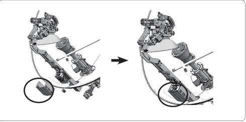
After arranging the cables, attach the Ku-band BUC Cover again.
