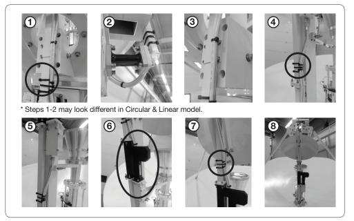
Ku Module Cable Arrangement (For a system with a BUC or EL Arm or Skew)
