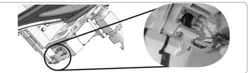
Connect the Waveguide and Flexible Waveguide (For Circular only model)
