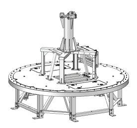
Preassembled Radome Base Frame The Radome base frame is assembled before it is put into the frame package.
