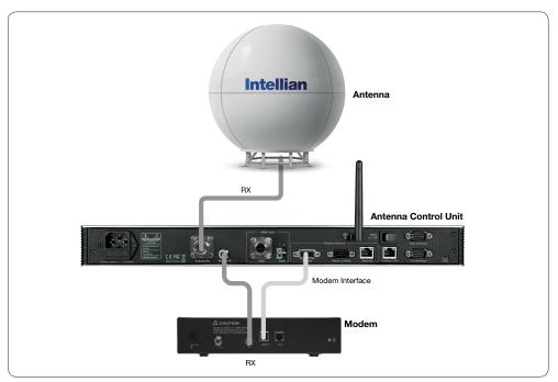
Basic System Configuration RX: 1 Antenna and 1 Modem
