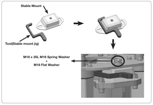
Fasten the Reflector and the Base Frame using M16x35L Hex Bolts
