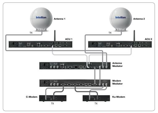
System Configuration TX: 2 Antennas and 2 Modems
