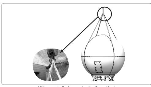
Lift up the Radome hanging all four straps on a crane hook as shown in the figure below. Straighten out the lifting straps as shown below prior to lifting the entire load of the antenna.
