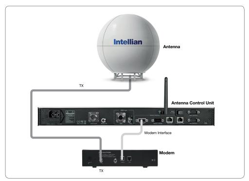
Basic System Configuration TX: 1 Antenna and 1 Modem
