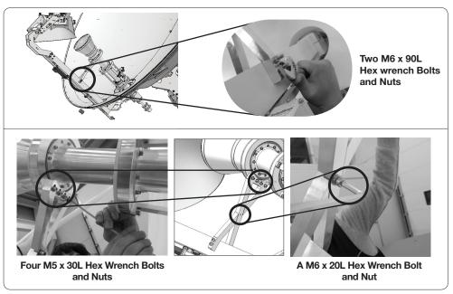
Assemble the Ku Module Support Frame and Feed Horn as shown in the figure below.
