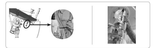
Ku Module Cables into the Reflector Hole
