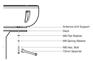
Figure 12: Mounting the Antenna
