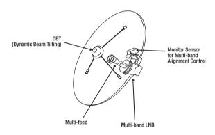
Figure 21: Multiband Alignment Control Systems
