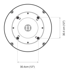
Figure 09: Mounting Hole Position of s6HD
