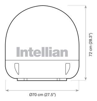
Figure 08: Radome Dimension of s6HD
