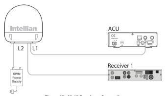
Figure 17 : Multi Receivers Connection
