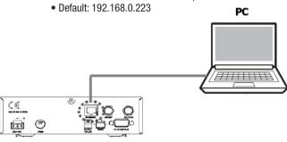
Figure 28: ACU to PC TCP/IP Connection
