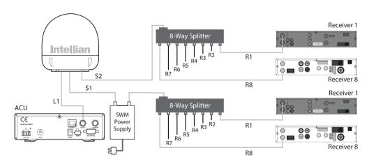
Figure 01 : Basic Configuration with 16 Receivers
