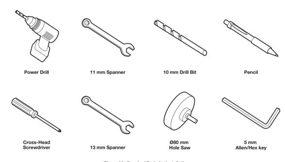
Figure 06: Required Tools for Installation
