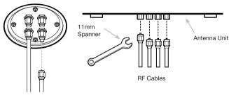
Figure 11: Connectors on Bottom of Antenna
