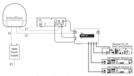
Figure 19: Multi Receivers Connection
