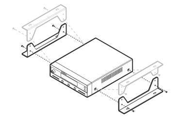
Figure 14: Mounting the ACU
