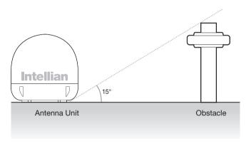
Figure 07: Elevation Limit of Obstacles
