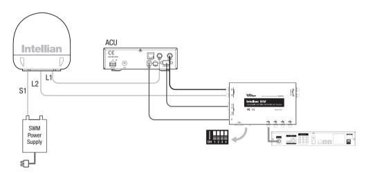
Figure 18 : Single Receiver Connection
