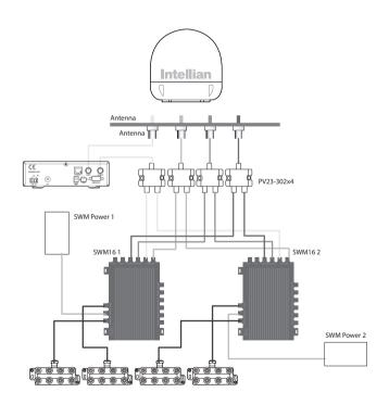
Figure 16: 32 Receivers Connection
