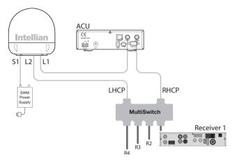
Figure 15: 16 Receivers Connection
