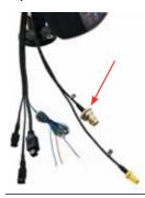
The antenna connections exit from the rear of the SatDOCK-G 9555 cradle, via the antenna loom as shown in the picture.
