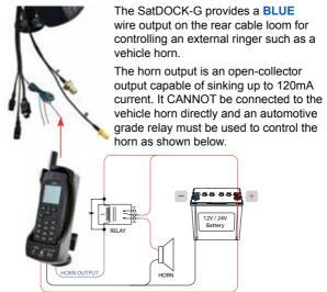
By default, it only works when the key ignition is OFF and the SatDOCK-G is still ON (by default, the SatDOCK-G will stay on for 20 minutes after the key ignition is turned OFF). This is to avoid the horn buzzing on an incoming call while the vehicle is being driven.
