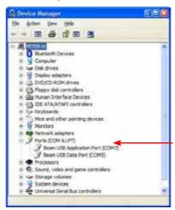
Please use the USB Data port for data communication. The USB Application port is used for SatDOCK-G 9555 configuration via the SDMS.
